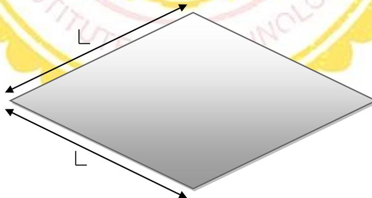
Fig. 1: Square plate simply supported on all four edges
