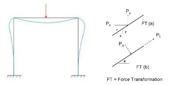
Suppose you are given the forces in FT (a) and you wish to transform these forces into Pn (normal) and Pt (tangential) as shown in FT (b). This force transformation may be necessary so that you can calculate the member axial and shear forces. These force transformations are summarized as
